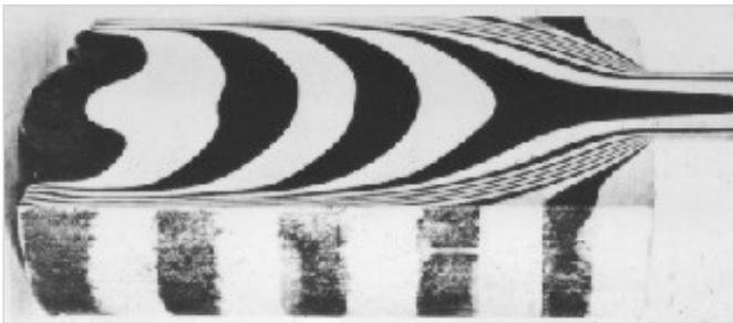
*As heated aluminum is forced out of the container and through the die, the core of the billet flows more rapidly than the periphery, as illustrated by the dark banding in this photograph. The periphery, which is left behind as residue, is recycled for future use.*
