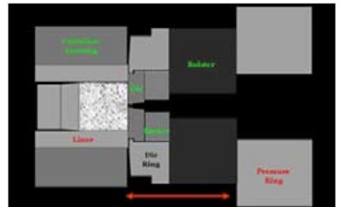
The ram piston/cylinder pushes the ram stem forward, which in turn pushes the billet through the container and then through the die (held in position by the die carrier) that ultimately forms the profile. See labeled illustration above (middle) that identifies the component parts involved in this process.
