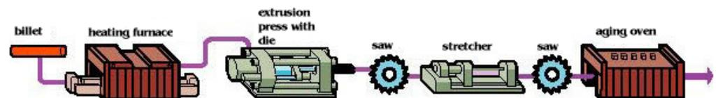
Once the shape of the final product has been identified, the proper alloy selected, and the die prepared, to make ready for the actual extrusion process, the billet and extrusion tools are preheated. During extrusion, the billet is still solid, but has been softened in a heating furnace. The melting point of aluminum varies with the purity of the metal, but is approximately 1,220° Fahrenheit (660° Centigrade).
