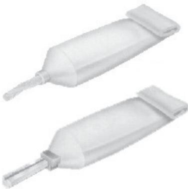
*As suggested by these toothpaste tubes, the shape of the extrusion (profile) is determined by the shape of the opening (die).*
