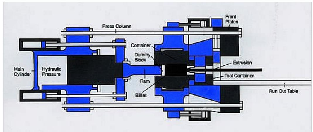
*This is a simple diagram of a typical horizontal hydraulic extrusion press; the direction of extrusion here is from left to right.*
