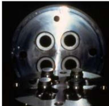
The most common types of hollow dies are the porthole and pancake. They typically are the most cost effective and easiest to manufacture, allowing the designer to be much more creative
