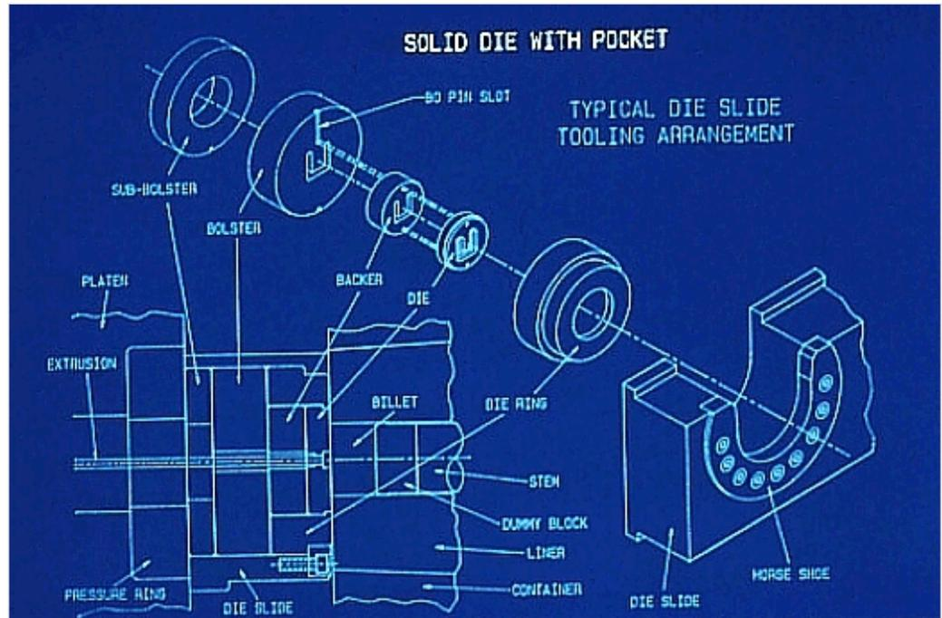
*This diagram shows the components that typically make up a die slide, the tooling assembly, for a solid die.*
