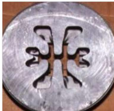
While a solid or semihollow die is a single piece, it requires support from additional tools called backers and bolsters. Depending on the complexity of the extruded shape, the total cost of the extrusion tooling may include charges for these supplemental tools.
