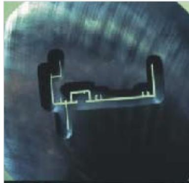
Solid dies may, on occasion, be used to produce hollow profiles by means of a fixed or floating mandrel. The use of a mandrel for extruding a hollow shape through a flat die usually involves the use of hollow billets, cylindrical source stock that may have been cast or bored. Piercing mandrels, however, do not require the use of cored billet.
